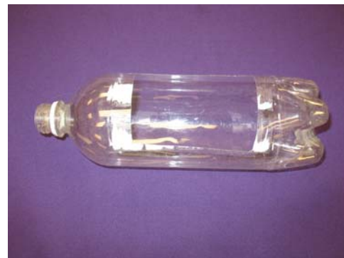
One-liter bottle with rectangular approximately 1/3 section cut out.
